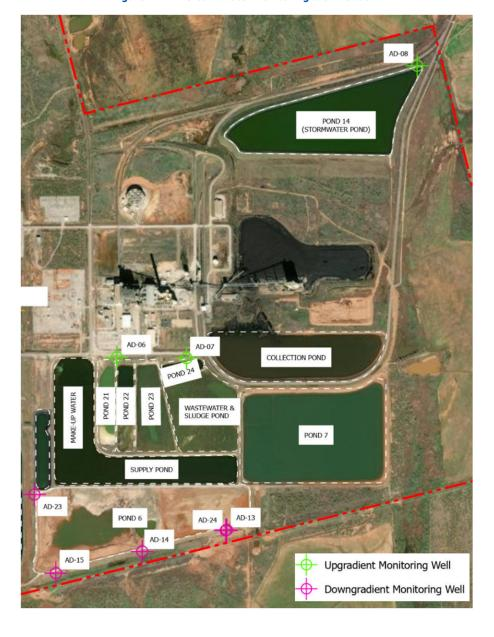
Figure 1-1: Groundwater Monitoring Well Network
